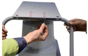
2.Tighten 4 screw of foot pedal from down side
