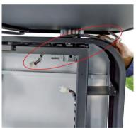
2. Put the power cord of the table from under the table into the chamber, like show in the picture.
